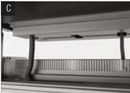
Cable routing from cable tray into CPU box.
